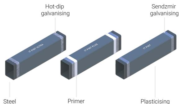
All finishes have a nanotechnological passivation layer between the steel and the primer or plasticiser.
